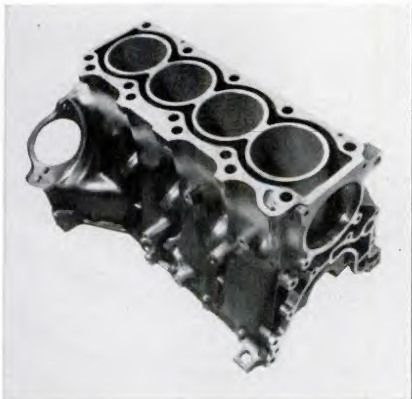
DOMESTIC FOURS include 2300-cc, aluminum-block (left) Vega engine. With overhead camshaft design (right), engine is available at 90 hp with single-barrel carb, or at 110 hp with double-barrel configuration
